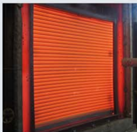
During fire test
